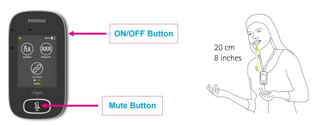
Switch on the Passaround mics via the ON/OFF button on the side - press and hold until you see the LEDs illuminate.
