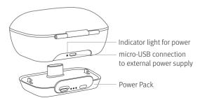
micro-USB connection to external power supply
